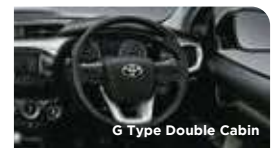
STEERING SWITCH (AUDIO, TELEPHONE, VR, MID) Steering wheel designed for excellent operability, incorporating control switches for audio, telephone, VR, and MID. (V & G Type Double Cabin)
